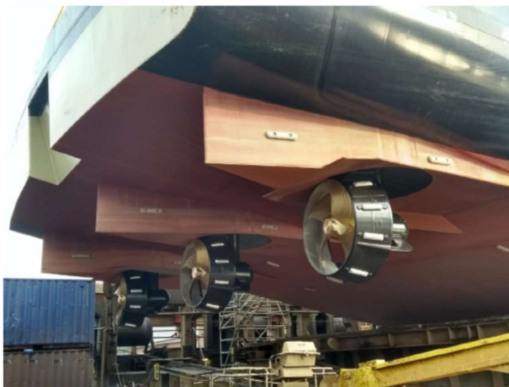
Figure 14: Aft ship design with 3 thrusters, reducing propeller diameter for low water operation (Source: MARIN, Photo: S. Oudakker, Oudcomb)
