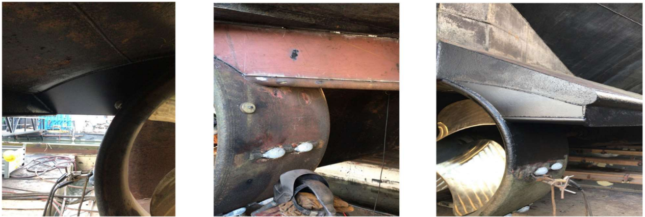
Figure 12: Optimisation of vessels' aft and propellers (Source: CONTARGO)
